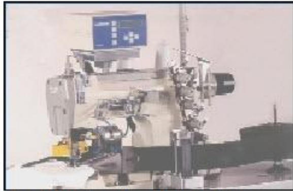
The EMX-2 is shown here with a PX Cutter mounted behind the needle
